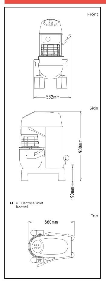
Electric Supply voltage: 200-240 V/1N ph/50/60 Hz **Electrical power max.:** 1.01 kW **Total Watts:** 1.01 kW Capacity: Performance (up to): 6 kg/Cycle Capacity: 20 litres Key Information: External dimensions, Width: 521 mm External dimensions, 685 mm Depth: External dimensions, Height: 980 mm **Shipping weight:** 87 kg Net weight (kg): 76
